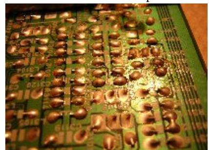
Lead Free joints of DIL IC Socket at Lower temp. 250deg
