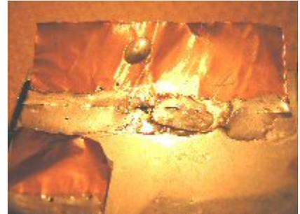
Copper plate joint with lead free & leaded solder
