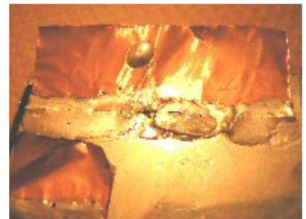
Copper plate joint with lead free solder
